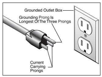
Figure 2. Typical type 5-15 plug and receptacle.
